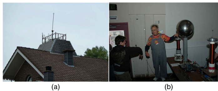
Figure 18.37 (a) A lightning rod is pointed to facilitate the transfer of charge. (credit: Romaine, Wikimedia Commons) (b) This Van de Graaff generator has a smooth surface with a large radius of curvature to prevent the transfer of charge and allow a large voltage to be generated.
